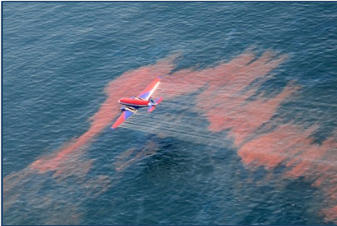
Aerial application of dispersants on surface oil. Photo courtesy of The Encyclopedia of Earth .
